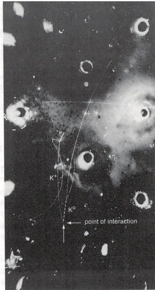
Fig. 6.8. “Muonless” Gargamelle neutrino event in which a K^+ meson and \Lambda^0 hyperon are emitted, and nothing else
